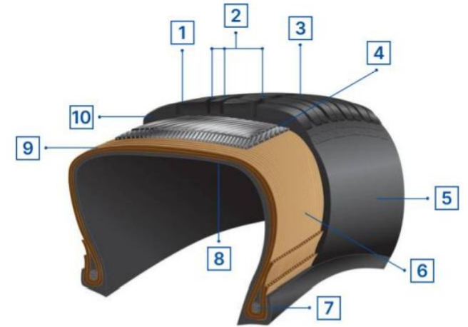
Figure 4-2: Schematic construction of a radial tyre.
